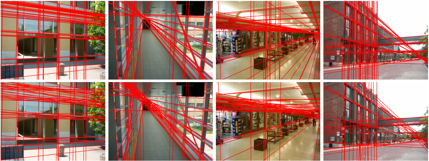
Fig. 5. Sample detections for the proposed framework (top) and Hough transform+NMS (bottom). The \lambda and \tau parameters were set so that both methods detect on average 50 lines per image. Note, how the proposed framework is able to discern very close yet distinct lines, and is in general much less plagued by spurious detections (please, zoom into the areas containing many near-parallel lines to observe the difference between the methods).
