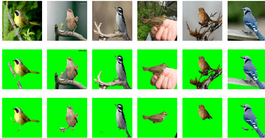
Fig. 4. More Bird segmentations: (top) original images, (middle) BiCoS outputs, (bottom) TriCoS outputs. The most noticeable difference between BiCoS and TriCoS is the removal of tree branches of leaves. These often appear in many images in one category, so that BiCoS segments them as foreground. But they appear across categories as well and are therefore not class-discriminative and are discarded in TriCoS.
